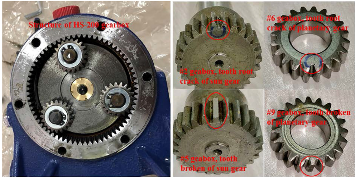
Fig. 3. Structure of the HS-200 planetary gearbox and 4 example damaged gears.
